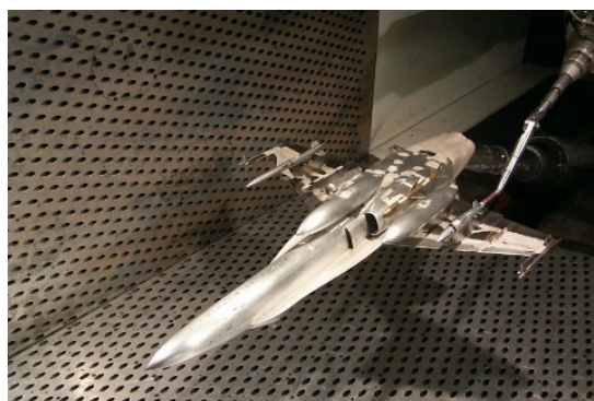
Figure 3: CTS Wind Tunnel Test.
